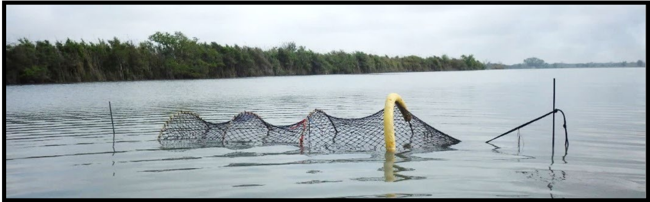
Figure 6 Example of hoop trap set in open water. Trap secured with rebar at front and back ends, floatation device (pool noodle) visible on right-most hoop of trap.
